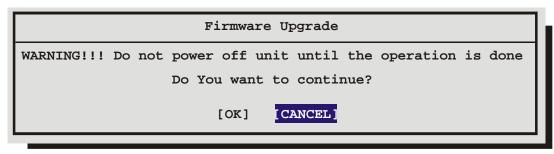
Selecting [OK] will put the DSR-1000eZ into Firmware Upgrade mode. The unit may now be programmed using WinFlash. The Operation may be cancelled by powering off the unit, as long as WinFlash has not started.
